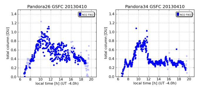
Figure 2: Total NO2 columns from Pandoras 26 and 34 at Goddard Space Flight Center (GSFC) on 10 April 2013 as a function of local time. Dark blue dots have passed the cloud filter. Light blue dots have not passed it. Pandora 26 data show rather large instrumental scatter from approximately 10:00 to 16:00, while Pandora 34 data show the natural variability only.
