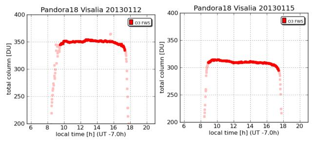
Figure 5: Total O3 column derived by Pandora 18 at Visalia, California, USA, on 12 and 15 of January 2013 as a function of local time. Dark red dots have passed the cloud filter; light red dots have not passed it. For air mass factor >5 (data before 9:15 and after 17:00) the instrumental stray light produces a negative bias in the derived O3 columns.
