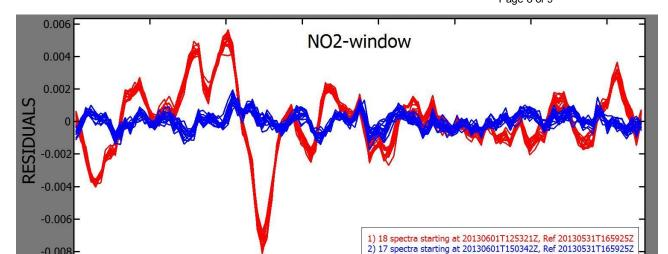
Figure 4: Residuals from NO2 spectral fitting for Pandora 23 for groups of spectra on 2013-6-1 as a function of wavelength for the range 426 to 441nm. Blue lines are spectra taken around 15:00 with RMS around 5e-4, i.e. the expected value. Red lines are spectra taken around 13:00 with RMS around 2e-3. The additional spectral signal for other spectra with elevated RMS seen in figure 3 also looks like the red lines.
