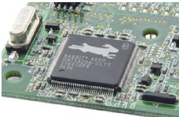
Figure 21: RabbitCore RCM4100 controller with up to 40 GPIO (General Purpose Input/Output), 59 MHz – 512K Flash, 256K / 512K Data SRAM (Static random access memory), 8 channels 12-bit A/D converter, Up to 6 CMOS-compatible serial ports
