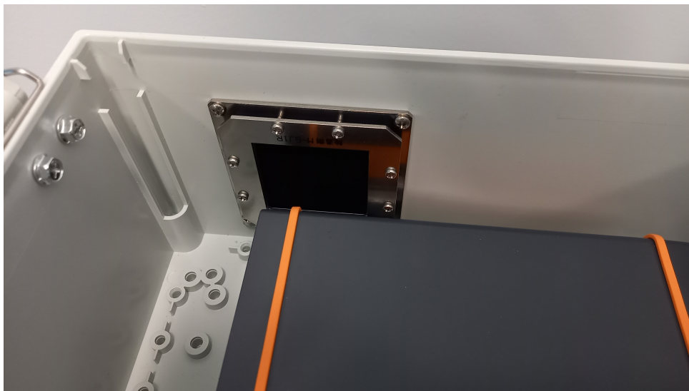
Figure 9: Inside of Pandora 234 spectrometer box with the dehumidifier installed.
