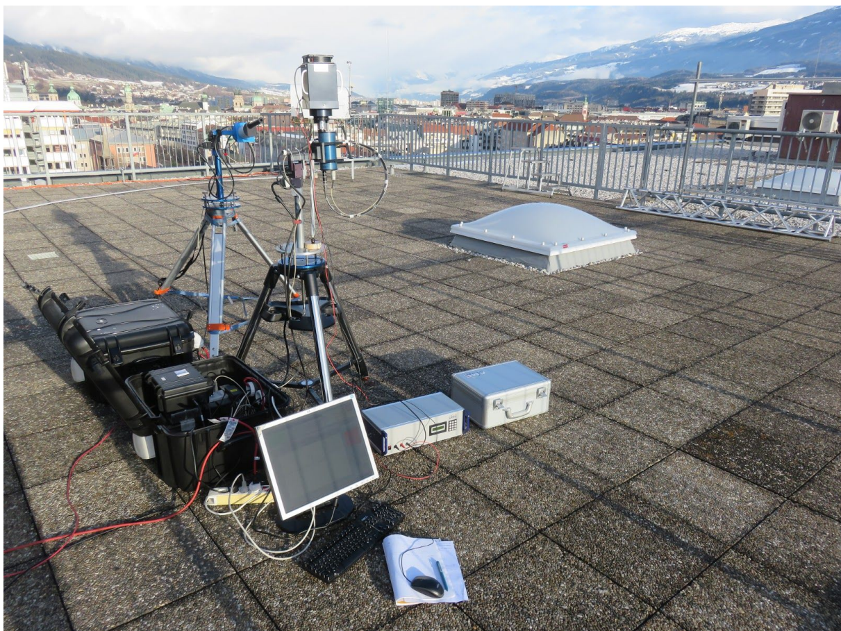
Figure 9: Pandora 106 on the Innsbruck Atmospheric Observatory with the final mFCT prototype. In the background one can see Pandora 119 which is being tested before shipping it to Athens. Right next to the screen there is the power supply for the lamp and right to it is the suitcase in which the lamp with the housing is stored.
