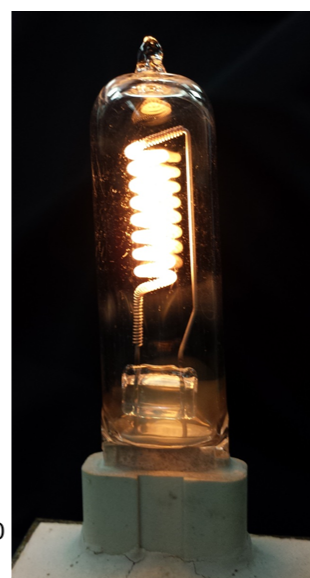
Figure 1: Right panel: picture of FEL lamp as used for the Pandora calibration. Left panel: spectral irradiance of FEL lamp running at 1000 W at 50 cm distance from the lamp.
