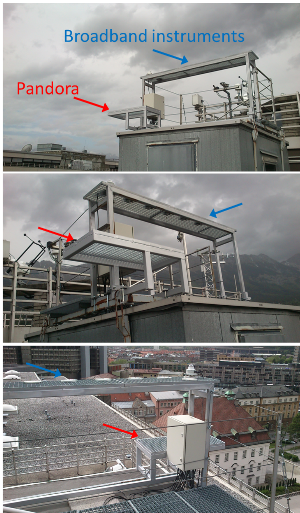
Figure 1: Pictures of the observation platform of the Biomedical Physics, Medical University Innsbruck. The Pandoras will be installed at the lower base (red arrow), so that the Pandoras head sensor is at the same height as the broadband instruments (blue arrow). Top panel is view from South-East. Middle panel is view from South-West with the mountain chain Nordkette in the background. Bottom panel is view from North
