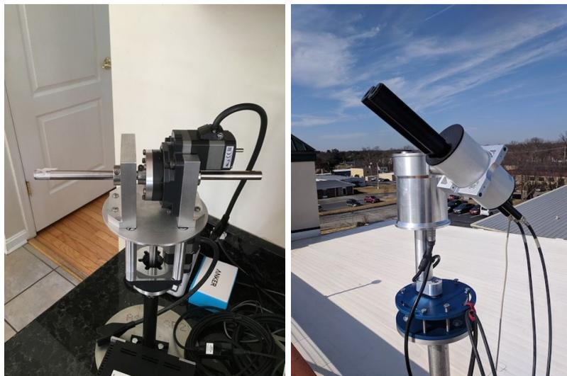
*Figure 1: Tracker prototype without sealed enclosure (left panel) and with enclosure and the Pandora head sensor (right panel).*
