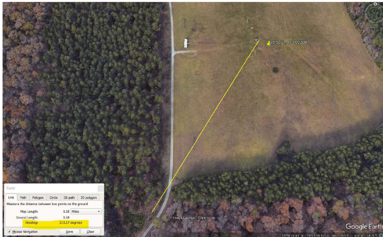
Figure 3: Example of an overview photo at site Chapel Hill, NC with a line drawn from Pandora to a clearing confirmation no obstructions of the determined Sky Scan Angle.
